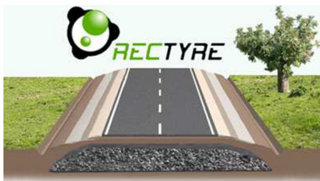
Figure 1: Embankment Shred Tire, Rectyre design scheme.
