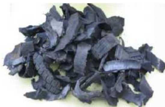
Figure 5: Tire shred in pieces ranging from 20 to 40 cm.
